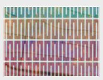
Organic solar cells require precise energy input during processing. The LPKF Proto-Laser U4 with a stable output power in the lower range can meet this requirement.
