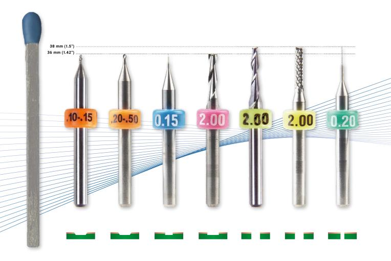
The tools are divided into two main categories: surface tools with a total length of 36 mm (1.42") for surface machining (cutters and end mills) and through-thickness tools with a total length of 38 mm (1.5") for penetrating the base material (spiral drills, contour routers, and end mills).
